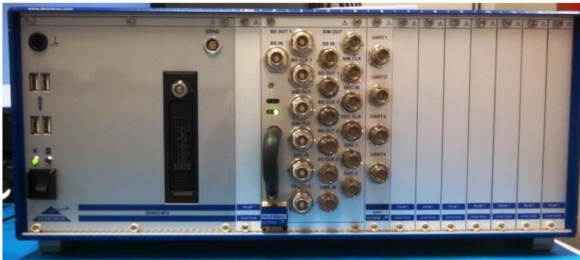
Figure 198 – Tarsus3 Panel Connectors in a cPCI Chassis
