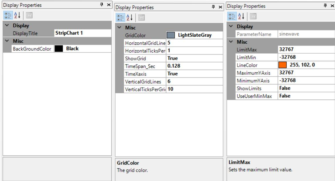
**Figure 120 – Three Display Property Windows for the Strip Chart Display**
