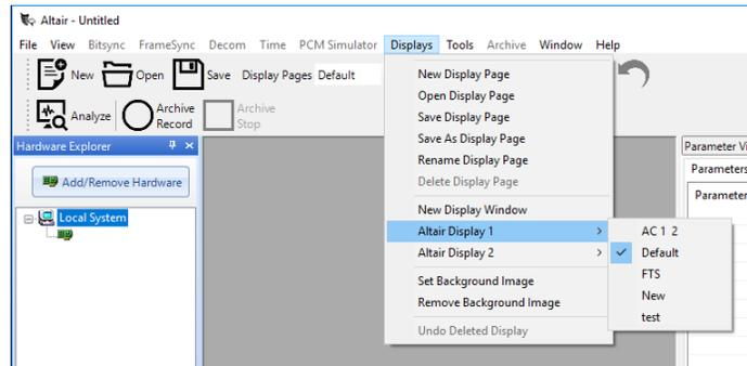
**Figure 87 – Selecting the Display Page for a Display Window**
