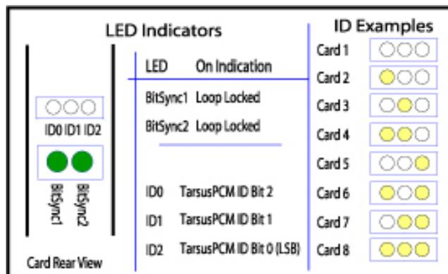
Figure 19 – LED Indicator Card Configuration Examples
