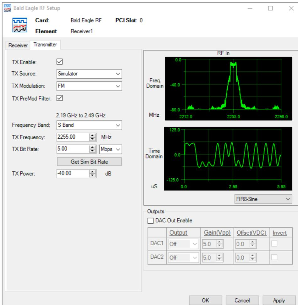
Figure 189 – Bald Eagle RF Transmitter Setup
