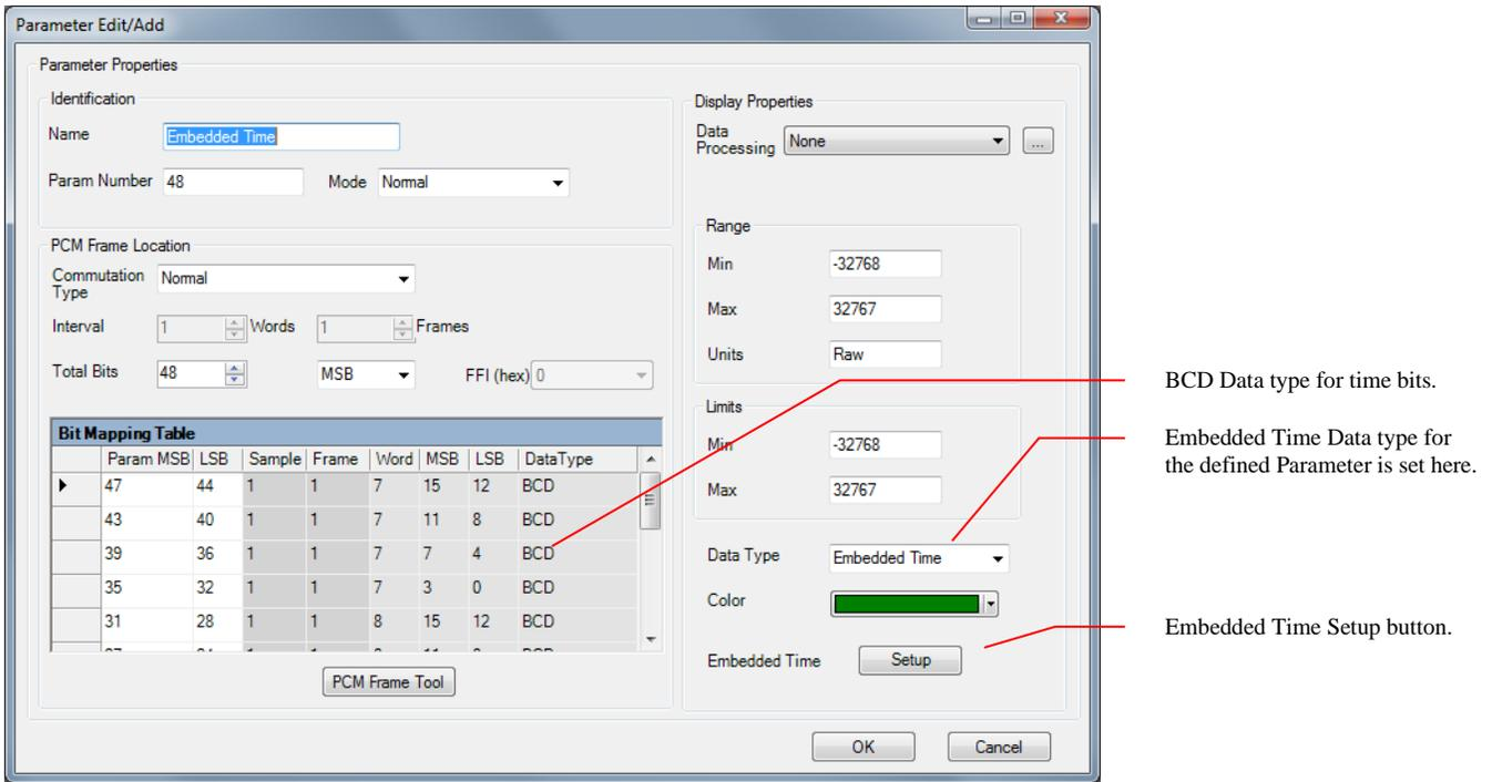
**Figure 132 – Embedded Time Parameter**
