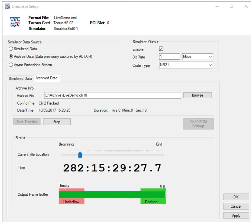
Figure 158 – Simulator Setup Window Chapter 10 Archive Simulator
