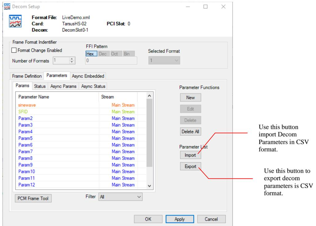
**Figure 67 – Decom Parameter Import / Export in the Decom Setup Window**
