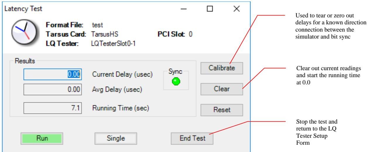
Figure 175 – Latency Test Form
