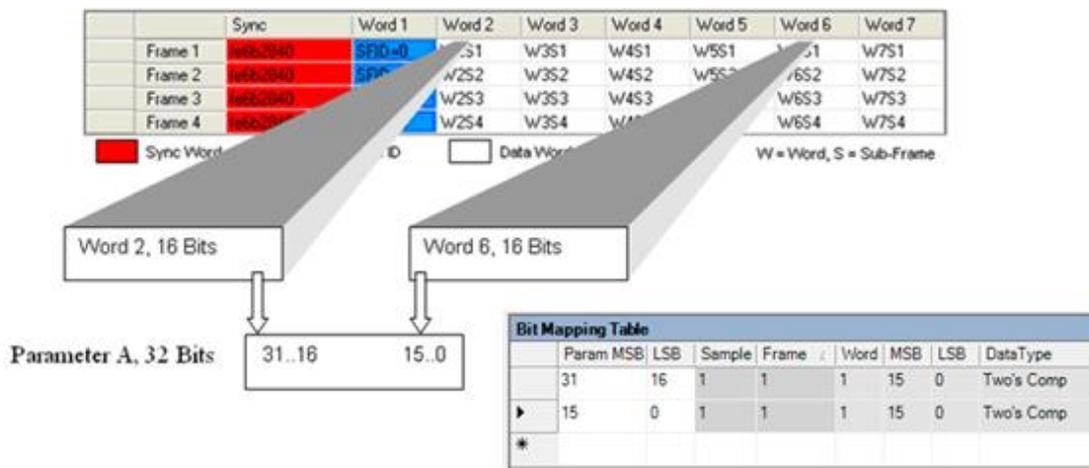
Figure 62 – Example of a 32-bit Parameter Created from Two 16-bit PCM Words
