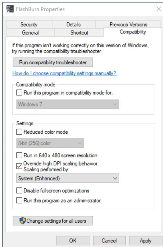
**Figure 205 – FlashBurn Windows 10 Override high DPI Scaling Behavior**
