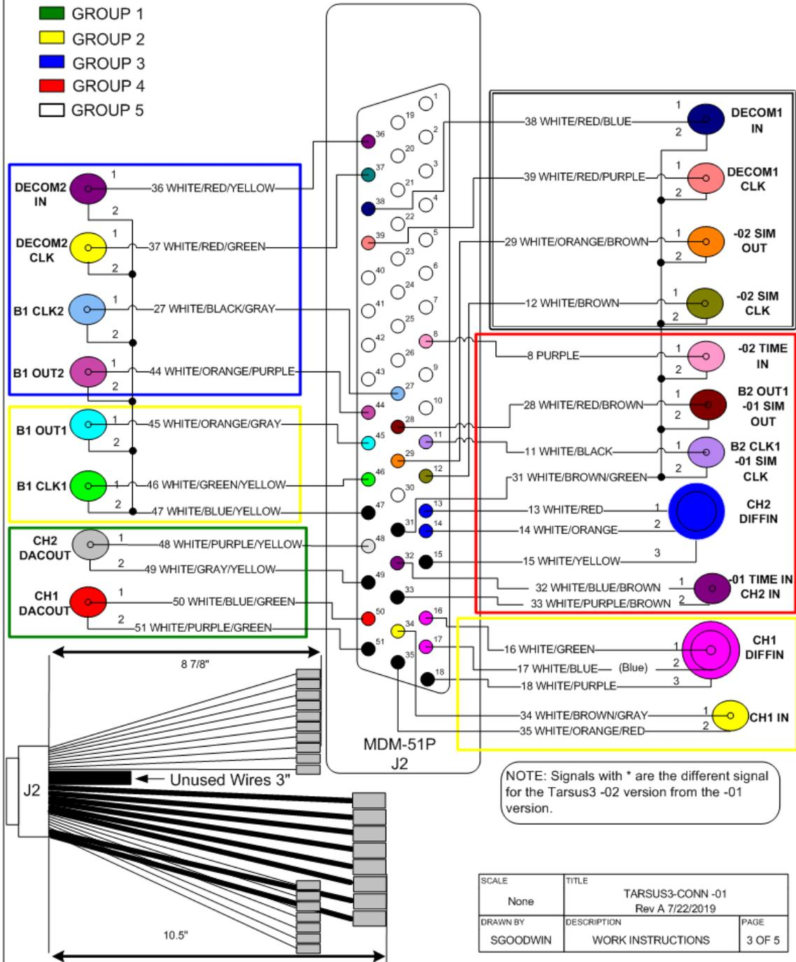
Figure 199 – Tarsus3-02/-01 Connector Diagram Part 1
