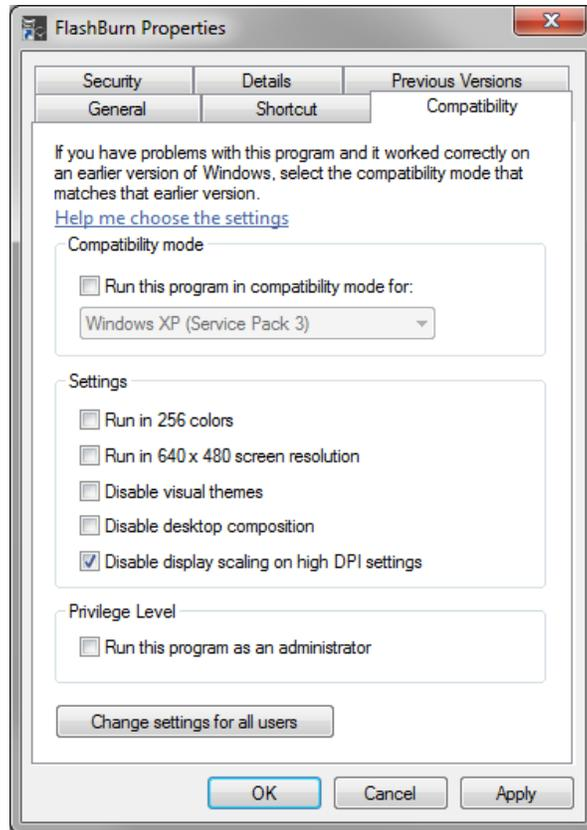
**Figure 207 – FlashBurn Windows 7 Disable Display Scaling on high DPI Settings**
