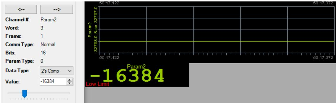
**Figure 185 – Channel Control Form Value of -16384 and Low Limit Violation**
