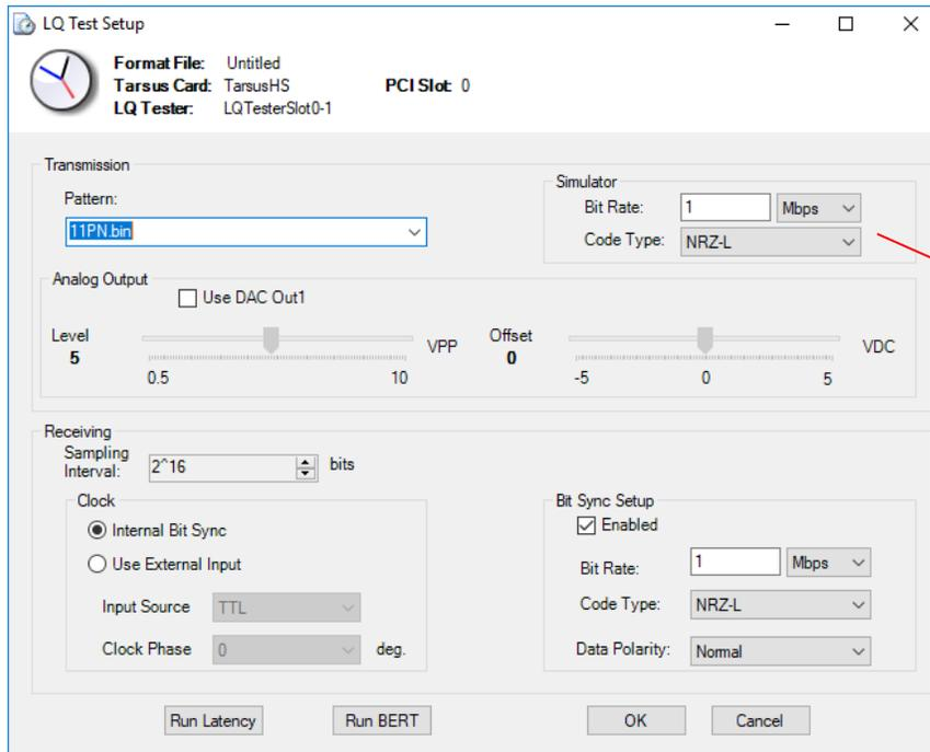
Transmission setup section of the LQ Tester
