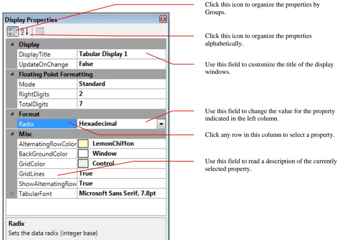
Figure 91 – Example of a Properties Window
