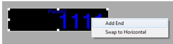
**Figure 105 – Add Additional Decom Parameter to Meter**
