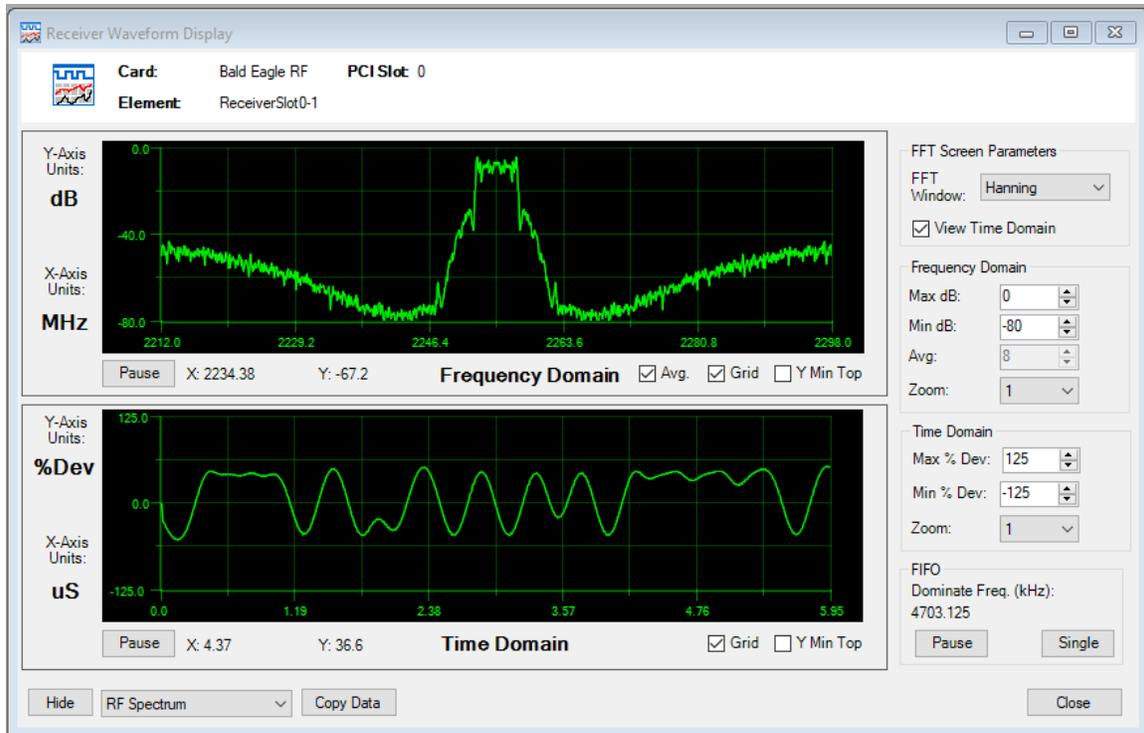
**Figure 82 – Bald Eagle RF Receiver Waveform Window**
