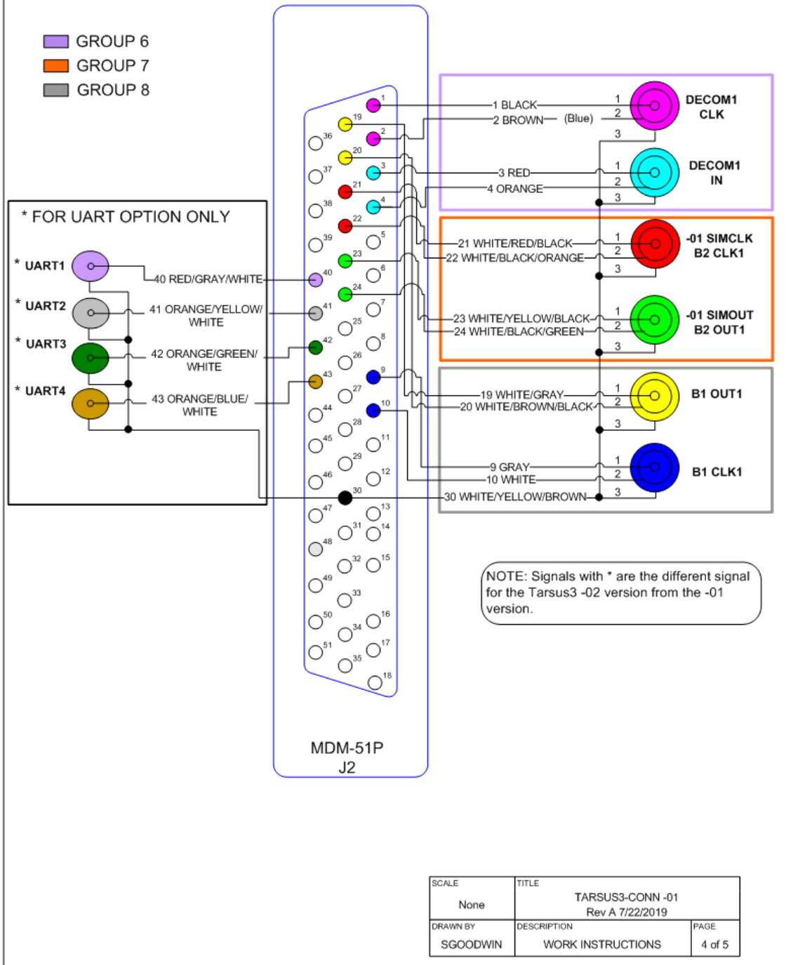
Figure 200 – Tarsus3-02/-01 Connector Diagram Part 2
