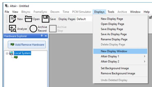
**Figure 86 – Display Window options in the Display Menu**
