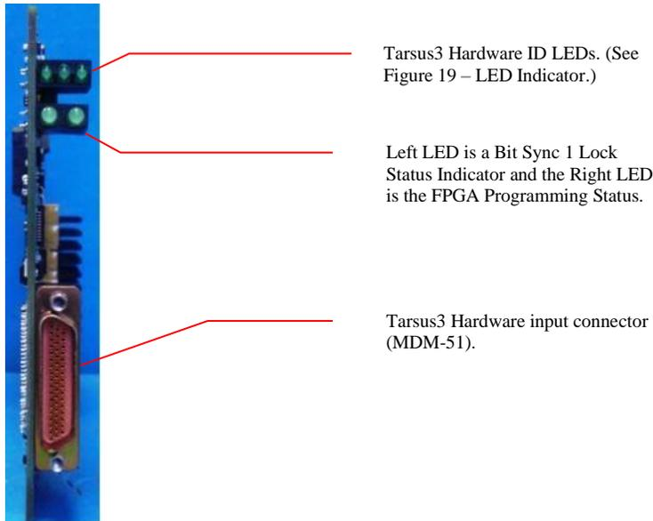
Figure 18 – Tarsus3 Rear Panel View of LED Indicators
