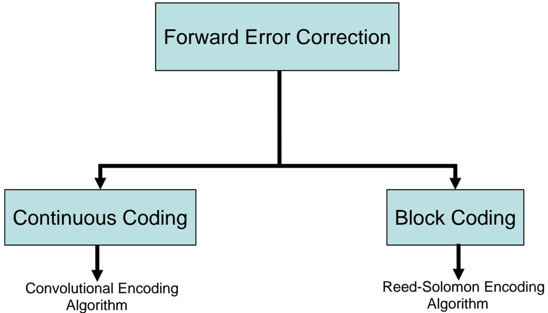
**Figure 210 – Forward Error Correction Block Diagram**
