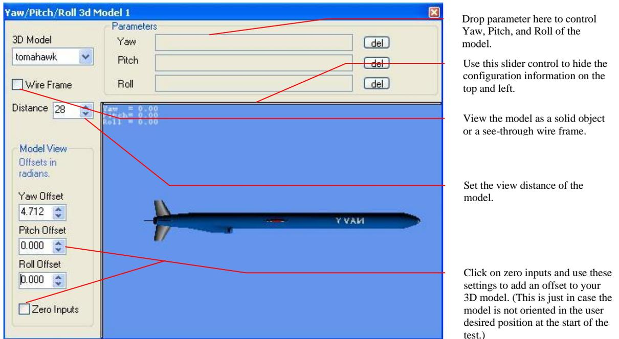
Figure 129 – 3D Model Data Display
