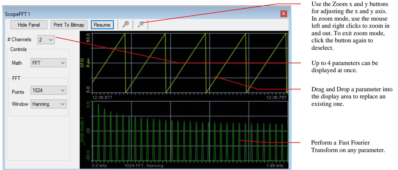
Figure 127 – Scope/FFT Data Display
